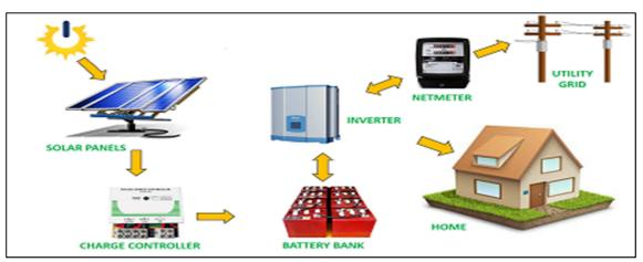
Generate power in the same way as a common on-grid solar system but use batteries to store energy for later use. This ability to store energy enables most hybrid systems to also operate as a backup power supply during a blackout, similar to a UPS system.
